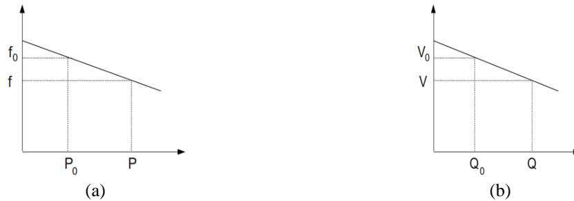
Figure 4. Droop characteristic of transmission line, (a) frequency droop and (b) voltage droop characteristics
